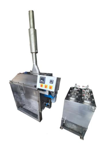
Polyglycol Heating chamber stainless steel double jacketed thermally insulated container,
