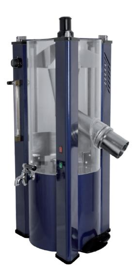
Usage : to study the de-inking effect of printed recycled paper by flotation method in laboratory.
