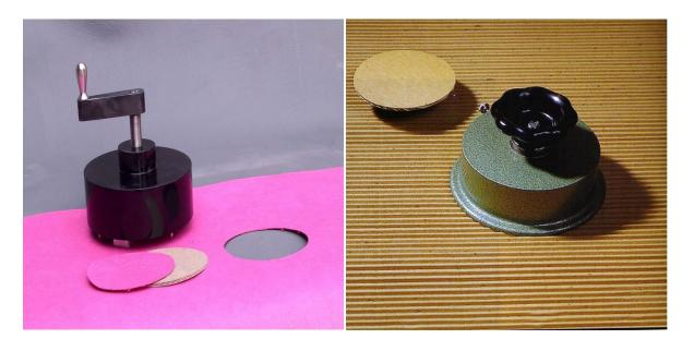
Usage: for the preparation of samples for the Flat Crush Test (FCT).
