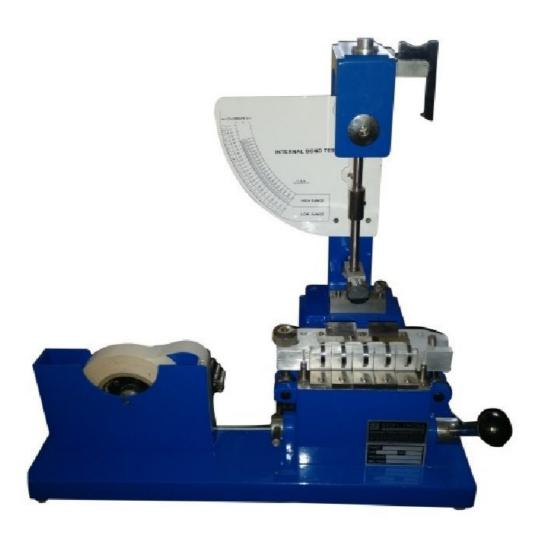
Usage: Determines the internal bonding of paper and board.
