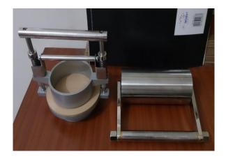
Usage: for measuring water or oil absorption of paper and board.
